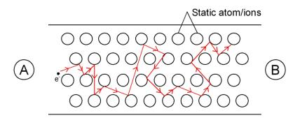
The figure illustrates the motion of a free electron within the conductor
