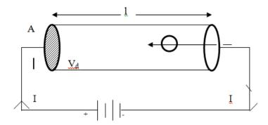
Consider the current in a conductor of cross-sectional area A.
